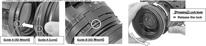
Once submerged, remove the lens underwater and shake it well to drop trapped bubbles especially from the rear lens surface then install the lens on the XD Mount again following same procedure.
